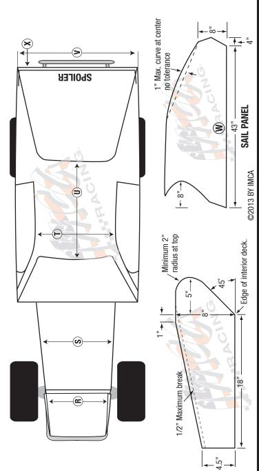
16" min. (ground to center of bumpers, front and rear) **B**—6.5" min. (center to center) A 23" max.
