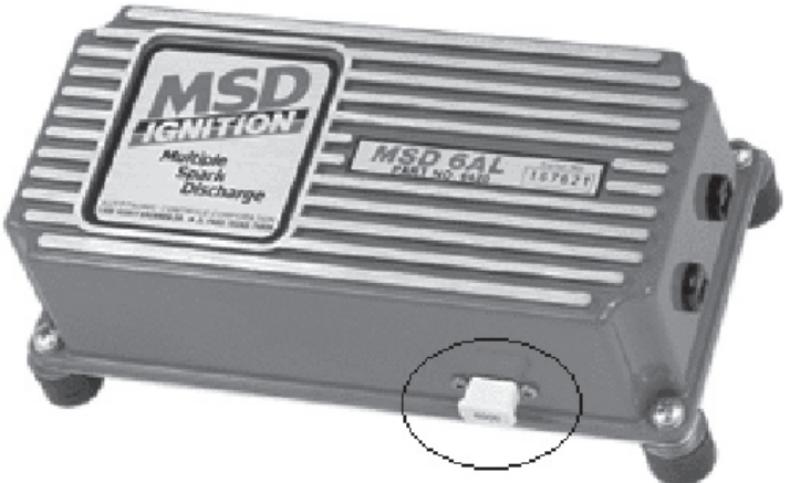
Location of the external chip on an MSD box
